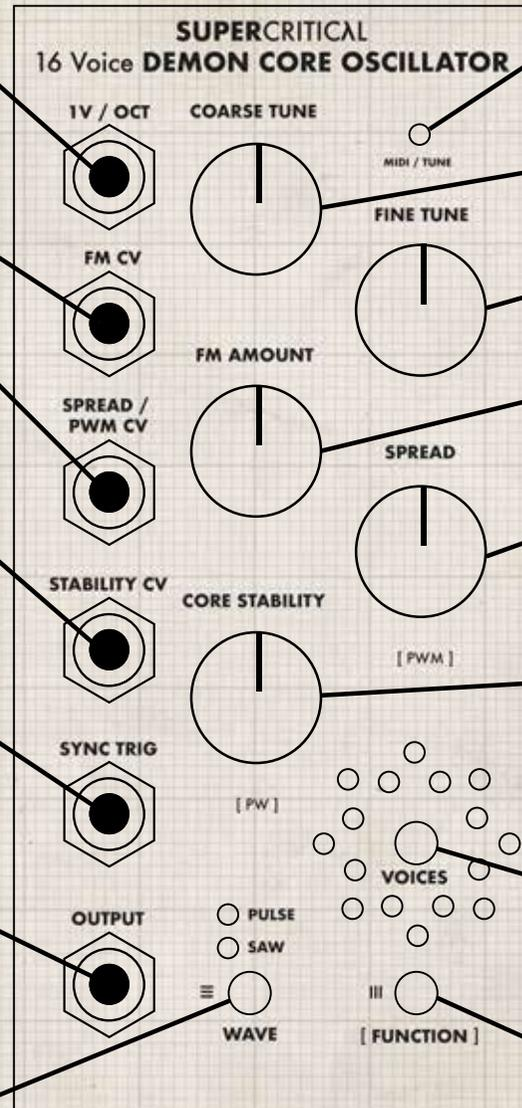
**MIDI/TUNE LED** indicates concert pitch when coarse and fine tune are rotated. It blinks on every C note (when there's no offset in **1V/oct**) and when fine tune is at center position for accurate tuning to A440. It also shows MIDI activity **when** expander is connected
